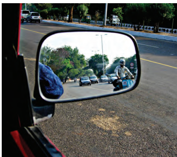
Fig. 15.20 Convex mirror as side view mirror
