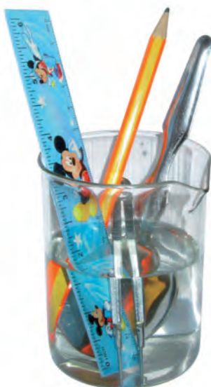
Fig. 4.8 Conduction of heat by different materials
