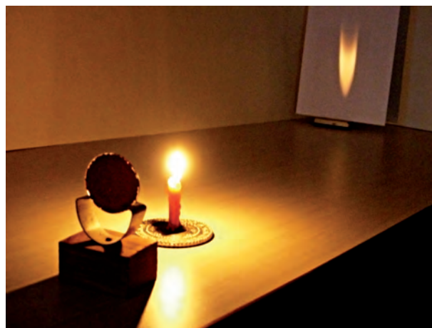
Fig. 15.15 Real images formed by a concave mirror
